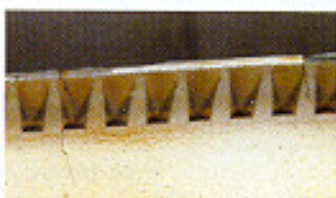
3, 4, 5. LPM powder metallurgy process repairs trailing-edge cracks (above); airfoil after blending to restore the original profile is at right
